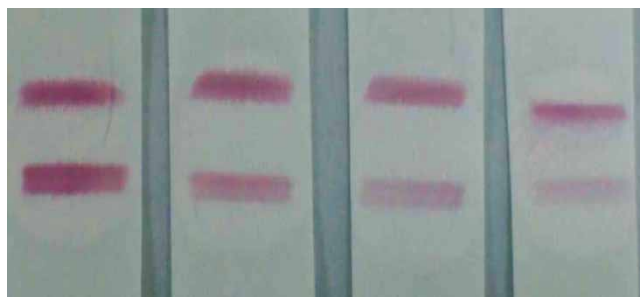
Figure 3. Lateral-flow immunogold assay. Top line: control line (goat anti-rabbit IgG); bottom line: test line (MPA hapten–OVA). MPA concentration from left to right: 0, 5, 10, 20 \text{ng g}^{-1} . The color intensity of 5 \text{ng g}^{-1} was clearly distinguishable from that of the negative control.
